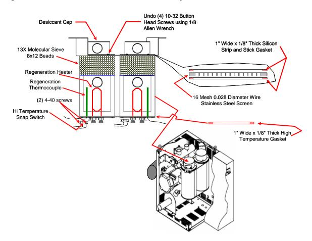
Figure 8: Desiccant Bed Location and Disassembly
